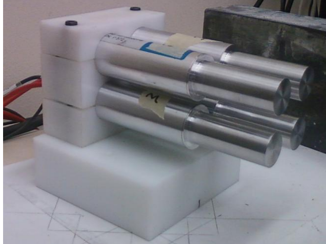
Figure 22. The detectors to be used for this detection system are Saint-Gobain manufactured BrillanCe 380 series 20mm x 51mm LaBr 3 (Ce) crystals with integrated PMTs. LaBr 3 (Ce) scintillator material is known for its exceptional energy resolution, fast emission and excellent linearity.
