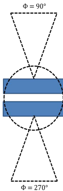
Figure 19. Shown are the conical backprojections expected from the geometry used for this project. No cones are projected to the right or left of the detectors in the figure.
