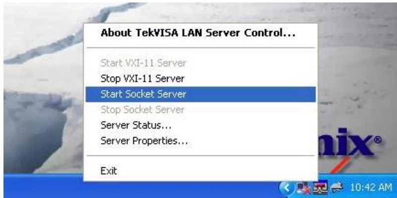
Figure 80. The first step to starting a TCP/IP connection between the oscilloscope and the host PC is to start the socket server. The location on oscilloscope to start the socket server is shown.
